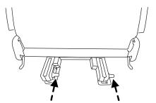
Do not place the seat front hooks on the front most pin of the front tub. Doing so will not allow the seat to fully install in vehicle.
